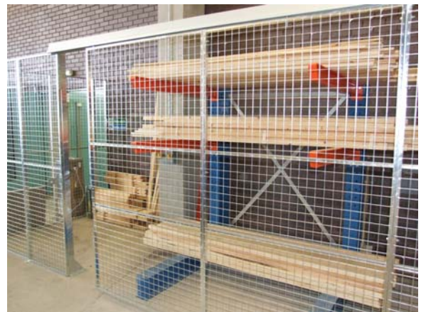
Cantilever shelving behind mesh
